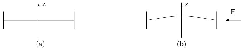
FIG. 9: (a): A flexible ruler is shown in its normal state as a horizontal straight line. (b): A certain force F is applied to push the ruler along its direction while its other end is fixed.
