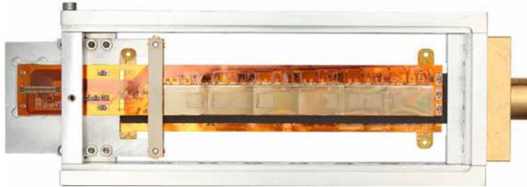
Figure 1: Front-view picture of the first full-size PLUME ladder hold in its test support frame. The connector appears on the left side, while the copper piece on the right is the air-inlet for the cooling.
