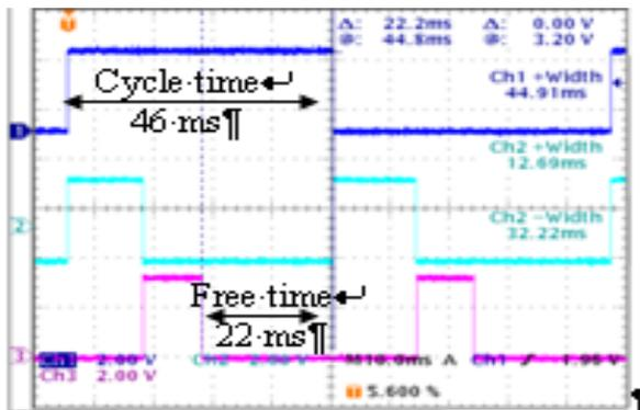
Figure 9 : CPU free time at full load (120 MB/s)
