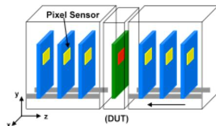
Figure 1 : Schematic view of EUDET Beam Telescope
