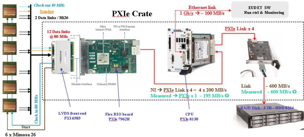
Figure 6 : EUDET Telescope DAQ based on PXIe Flex RIO architecture
