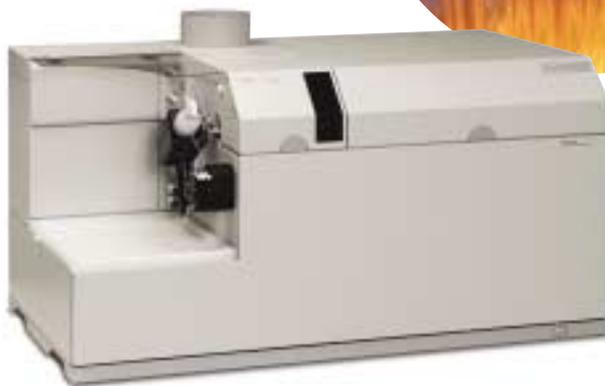
Many companies have already increased productivity and efficiency in their metals lab by replacing multiple techniques with a single Agilent 7500 ICP-MS. This trend has increased with the development of our ORS systems. With the widest dynamic range, coupled with freedom from matrix interferences, Agilent's ORS ICP-MS is replacing ICP-OES, GFAA, and elemental analyzers worldwide.
