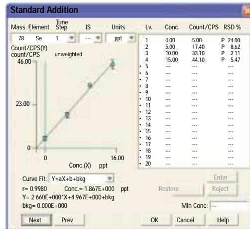
Standard addition calibration of Se using H<sub>2</sub> reaction mode showing good linearity even at 5 ppt. BEC is 1.9 ppt Se. While He collision mode can also be used for trace Se, H<sub>2</sub> mode offers unmatched performance.
