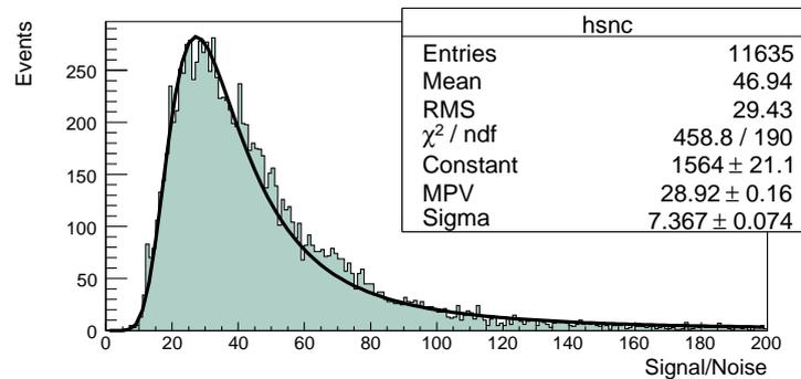
Fig. 1. Signal to noise ratio distribution for the seed pixel of hits produced by 120 GeV pions.
